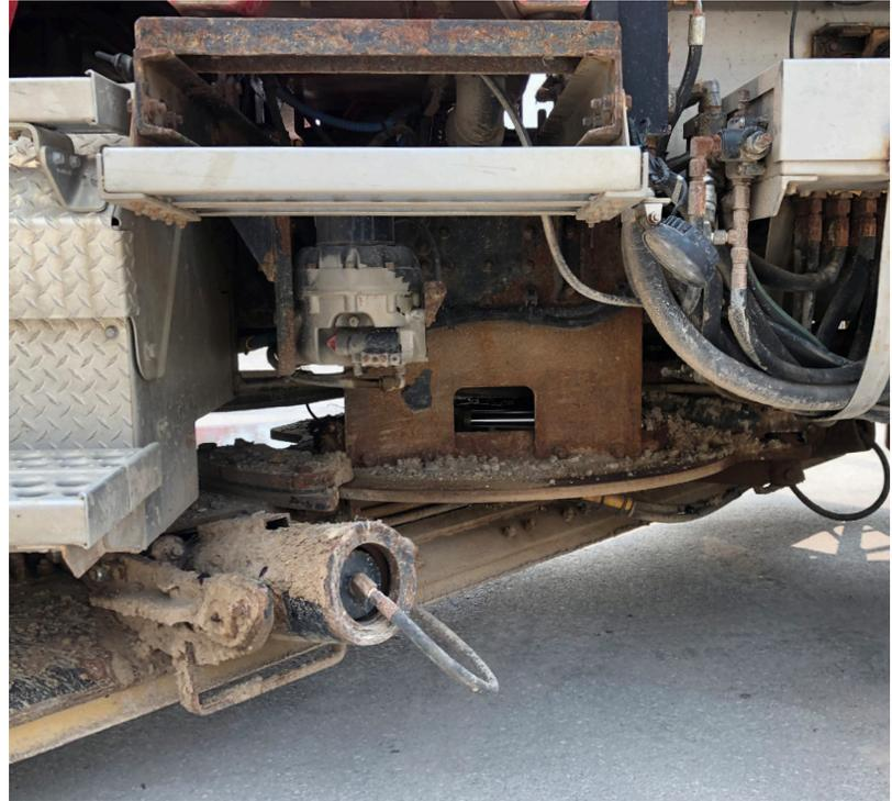
*"Since we have lots of plow and salt trucks, we are basically our own worst enemy. It was normal for frames to rot out, brake valves to corrode, the rear disk covers rot out, and even the transmissions. We needed a better way to flush and clean the trucks."*
